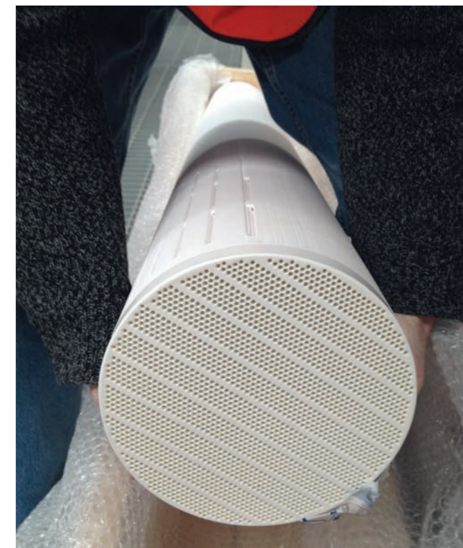
CeraMac vessel elements installed at Melbourne's Eastern Treatment Plant.
